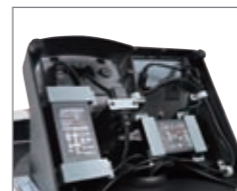
Separate Power Supplies for The Printer & Terminal
