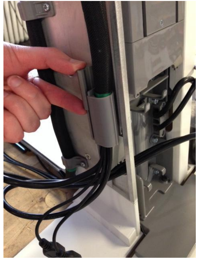
12. Slide the Clamp Sleeve onto the Dynamic Cable Clamp to fasten it.
